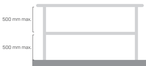
RAILING WITHOUT TOE BOARD
