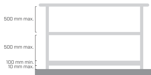
RAILING WITH TOE BOARD
